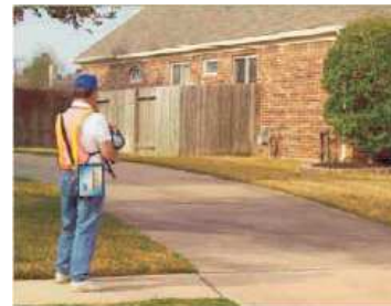
Safe Measurement: up to 30 meters away from the leak
