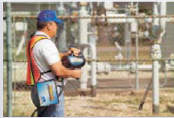
Detection & Pinpointing: RMLD, Gasurveyor
